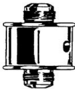
Carbonator Backflow Prevention
